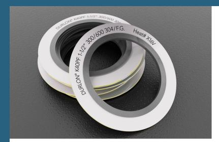
Durlon<sup>®</sup> Kammprofile gaskets have a solid metal core with concentrically serrated grooves machined into the top and bottom faces. The metal core is typically stainless steel, but it can be supplied in various metallurgies as per the customer's request.
