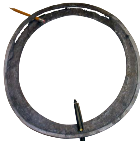
Cut almost entirely around the gasket at the OD of the raised face due to severe over-tightening (flange rotation).
