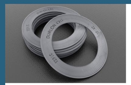
Durlon<sup>®</sup> CFG is a corrugated flexible graphite gasket material designed for severe service conditions. The proprietary design of the corrugations gives Durlon<sup>®</sup> CFG superior sealing and recovery characteristics for tough conditions in the refining, chemical, petrochemical, and pulp & paper industries. Durlon<sup>®</sup> CFG is suitable for service in steel, oil, mild alkalis, mild acids, hydrocarbons, and solvents.
