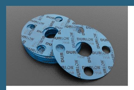
Durlon® 7950 is an economy grade general service gasket sheet material made with NBR (Nitrile Butadiene Rubber) binder for mild service in piping and equipment with applications in steam, hydrocarbons and refrigerants and an alternative when temperature and pressure conditions are below 500°F (260°C) and 1,200 psig (See PxT chart below for validation).
