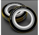
**Durlon® Spiral Wound (DRI FG SWG)** Gaskets are made with an alternating combination of a preformed engineered metal strip and a more compressible filler material which creates an excellent seal when compressed. The engineered shape of the metal strip acts as a spring under load, resulting in a very resilient seal under varying conditions.
