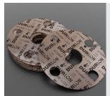
**Durlon® HT1000®** consists of phlogopite mica paper impregnated with an inorganic binder at less than half the binder amount found in vermiculite-phyllosilicate filled products. This lower binder content allows for superior weight retention, less than 4% weight loss at 800°C (1,472°F), and results in ultimate extreme temperature sealing performance up to 1,000°C (1,800°F).
