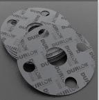
**Durlon**® **8900** is a premium grade material for service conditions to 496°C (925°F) and continuous operating temperatures of -40°C to 400°C (-40°F to 752°F). Suitable for saturated and superheated steam, oil, dilute acids and alkalis, hydrocarbons, and solvents.
